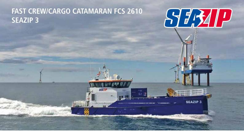
M.V. SeaZip 3 is a fast Twin Axe Bow catamaran for transport of personnel, equipment and parts to offshore windfarms, etc.
