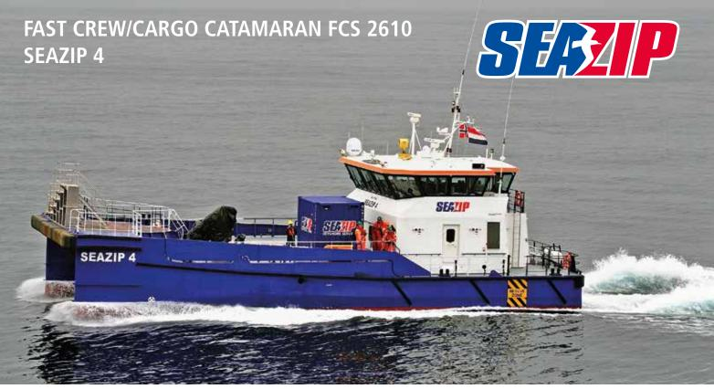
M.V. SeaZip 4 is a fast Twin Axe Bow catamaran for transport of personnel, equipment and parts to offshore windfarms, etc.
